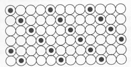
The above figure shows adsorption geometry of O on Pt{100}. Write down the Wood' notation and the matrix notation.
