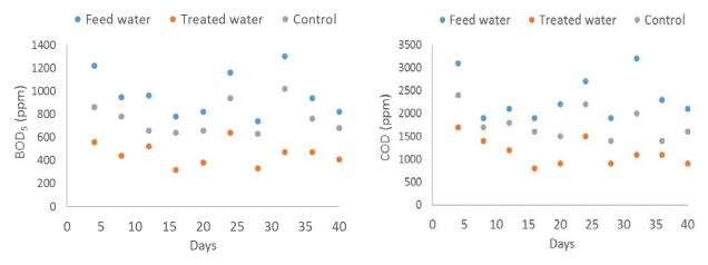
Fig. 3 Temporal change in organics removal (a) Removal of BOD<sub>5</sub> (b) Removal of COD
