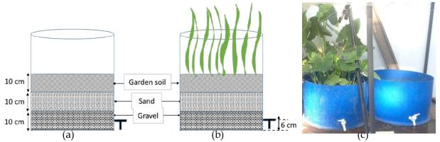
Fig. 1. Pilot scale vertical sub-surface flow constructed wetlands (a) schematic diagram of control (b) schematic diagram of experiment (c) real experiments both control and experiment
