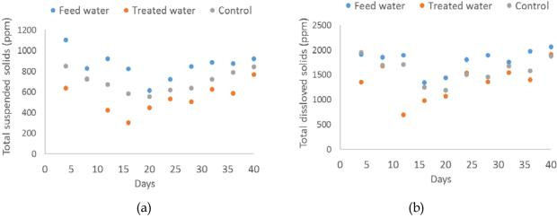
Fig. 2. Temporal change in the removal of solids (a) Removal of total suspended solids (b)
