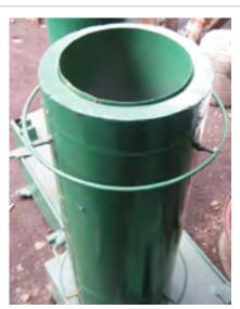
**Figure 2:** The gasifier reactor of inner diameter 20 cm, outer diameter 23 cm and height 0.6 m were made by Zn coated iron sheets. Use to store the rice busk
