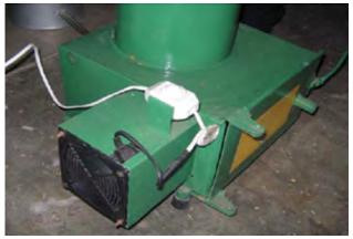
Figure 4: The air blowing system consist a control switch and DC (12 V-3 W) computer cooling fan to blow the air into the glasifier.
