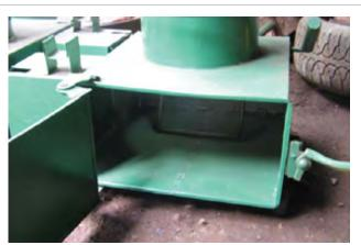
**Figure 3:** The char chamber of length: width: height is  $50 \times 50 \times 20$  cm. Which is the storage device of the end product.
