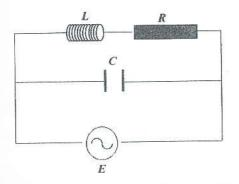
As shown in the above figure a coil of inductance L and resistance R is connected across the terminals of a capacitor of capacitance C and an alternating voltage  $E = E_0 \sin \omega t$  is applied across these same terminals.
