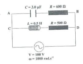
Consider the circuit shown in above figure. The amplitude voltage of the source and its angular frequency is 1000 rad.s<sup>-1</sup>. The values of the passive circuit eler shown in the figure. Determine
