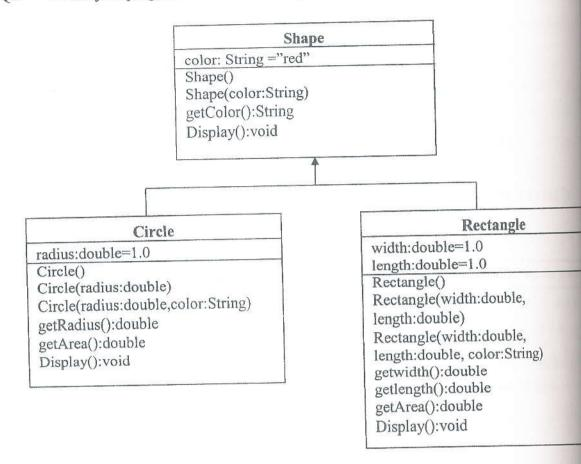
Create a super class called Shape (as shown in the class diagram), which contains:
