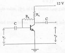
Figure shows a modified form of the simple Common-Emitter amplifier, where the base bias is supplied from the collector instead of the positive power supply terminal. The transistor has  $\beta = 100$ , and it is required to set the operating point such that  $V_{ce} = 6$  volt, and  $I_c = 1$  mA.
