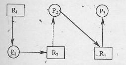
P<sub>1</sub>, P<sub>2</sub>, and P<sub>3</sub> are processes. R<sub>1</sub>, R<sub>2</sub>, and R<sub>3</sub> are resources.
