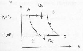
The Joule cycle shown above consists of two constant-pressure steps connected by two adiabatic. Show that the Thermal efficiency of a reversible engine operating in this cycle, with an ideal gas of constant heat capacities as the working medium is,
