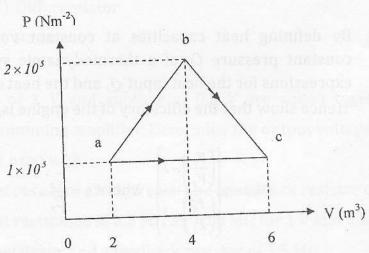
If a heat of  $8 \times 10^5$  J is added to the gas system along the path abc then find,
