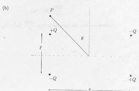
Four equal charge of magnitude Q as shown in figure are located as to form a quadrupole (double-dipole). Prove that if r is very much greater than l and s the potential due to this quadrupole is given by  $\frac{Qls\ sin2\theta}{4\pi\epsilon_0 r^2}$ .
