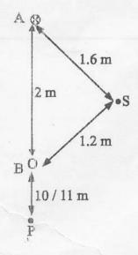
Two long straight parallel wires are 2m apart, perpendicular to the plane of paper. The wire A carries a current of 9.6A, directed into the plane of the paper. The wire B carries a current such that the magnetic
