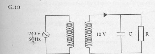
The figure shows a simple rectifier circuit. Sketch the out put signal when the
